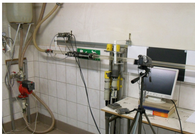
Figure 2. View of the measuring part of the hydraulic installation for liquid–gas flow tests in a horizontal pipeline.
