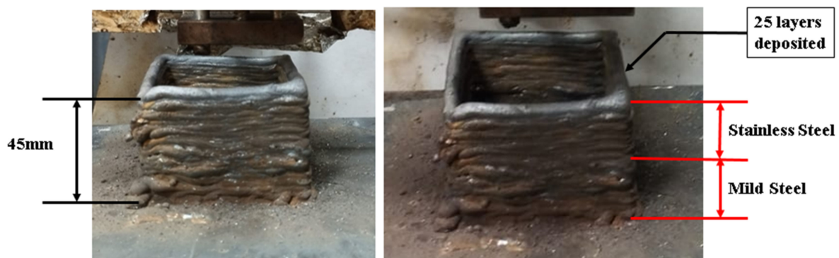
Figure 12. Mild steel and stainless steel bimetallic deposition.
