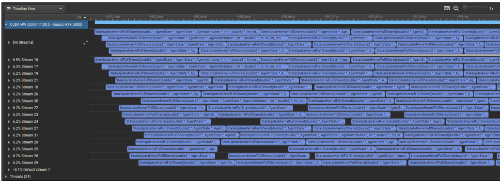
Fig. 12: NVIDIA Nsight Systems screenshot showing use of 16 CUDA streams.
