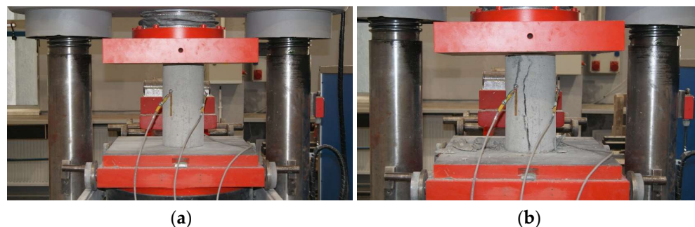
Figure 6. Concrete specimen at the time of testing: prepared for test (a) and after destruction (b).
