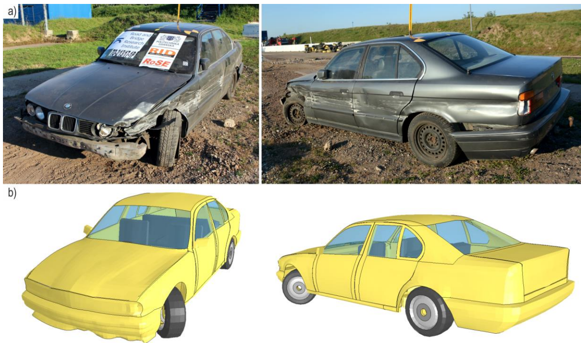
Fig. 14 Damage to the vehicle: a) crash test and b) simulation.
