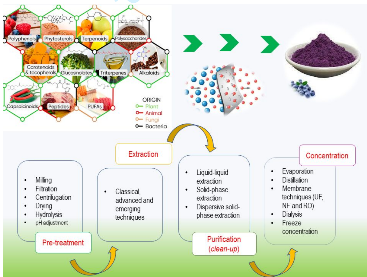
23 24 25 26 27 28 29 30 31 32 33 34 35 36 37 38 39 40 41 42 43 44 45 46 47 48 49 50 51 52 53 54 55 56 57 58 59 60 61 Figure 1. Main bioactive compounds extracted from natural sources and typical extraction 62 strategy required for their concentration. 63
