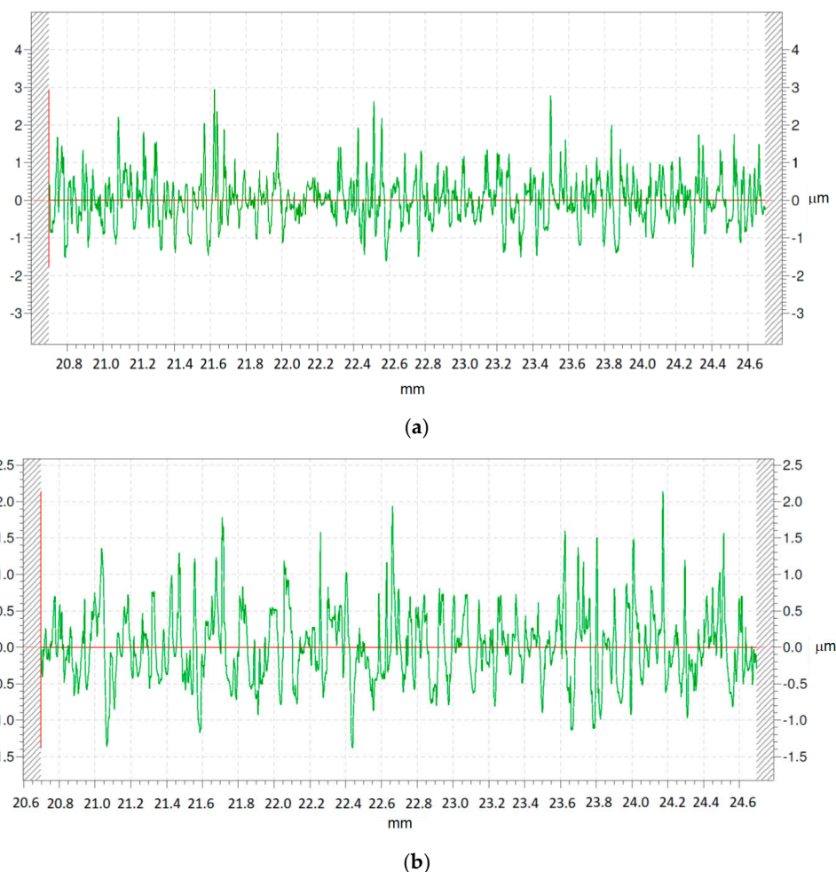
Figure 6. Roughness profiles of: (a) Experiment 9, obtained with high pressure of 600 \text{ N/cm}^2 ; (b) Experiment 11, obtained with low pressure of 400 \text{ N/cm}^2 .
