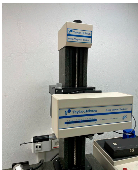
Figure 3. Taylor Hobson Talysurf 2 contact roughness meter.
