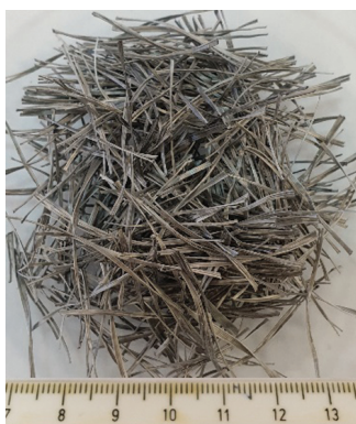
Fig. 3. Polymer fibers of a length of 24 mm
