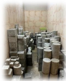
Fig.4: Curing the concrete samples.
