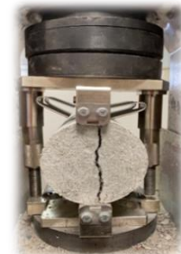
Fig.6: The splitting test.
