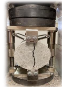
Fig.6: The splitting test.
