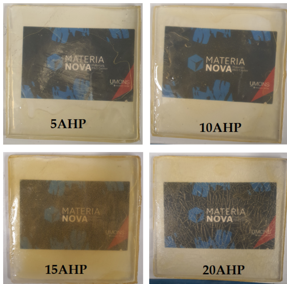
Figure 6. PLA plates surface coated with epoxy/AHP nanocomposite films containing 5, 10, 15 and 20 wt.% AHP nanoparticles.
