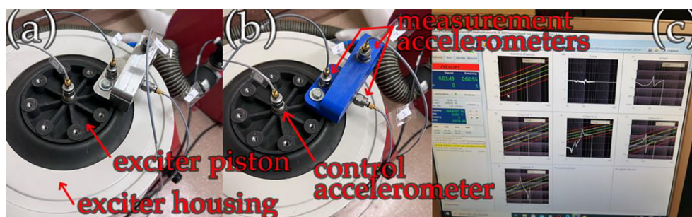
Fig. 7. Dynamic test course – mounting of piezoelectric sensors and the holder bracket on the vibration exciter: a) taking characteristics from the sample made of C35 steel, b) taking characteristics from the sample filled with 50% of filament, c) a screenshot with an image of the measurement programme – course of measurement curves /own elaboration/.
