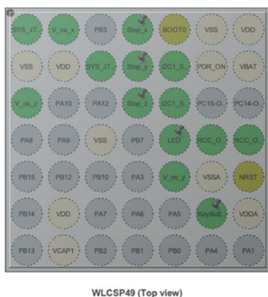
Fig. 13. Configuration of peripherals in STM32F411
