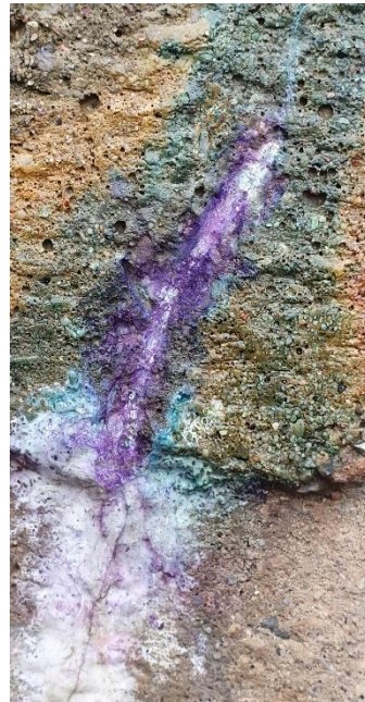
Photo 5: Discoloration of concrete after the Rainbow Test on the concrete surface, in the place of a crack on the wall of the right annex - test site after the test: a) view, b), c) close-up: green-violet coloration indicates advanced carbonation of concrete and its reduced ability to protect the reinforcement, the orange color indicates advanced carbonation of the exposed concrete surfaces, washing out of calcium carbonates is visible in the area of cracked concrete fragments
