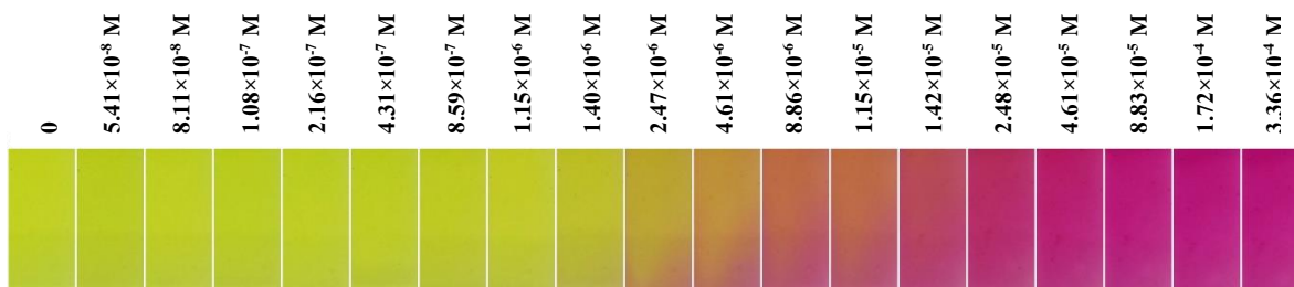
Fig. 23. Color changes of optode upon titration with copper(II) chloride ( c_{Cu} = 0-3.36 \times 10^{-4} M) at pH 5.0.
