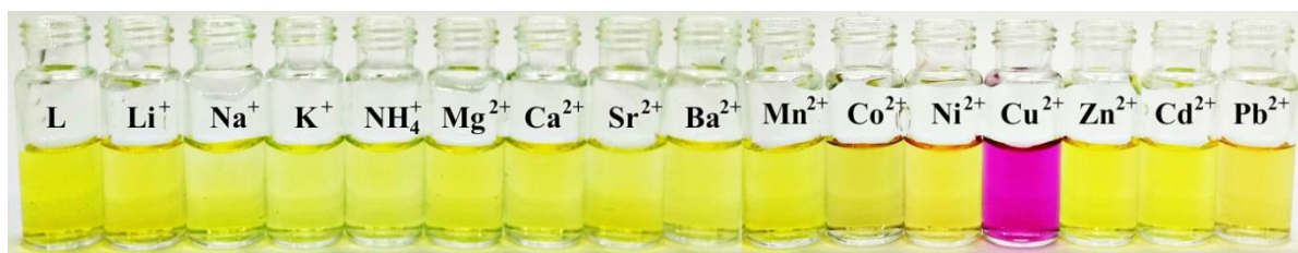
Fig. 13. Color change of ligand ( c_L = 2.16 \times 10^{-5} M) in water-DMSO solution (9:1, v/v) in the presence of metal chlorides (pH 6.0).
