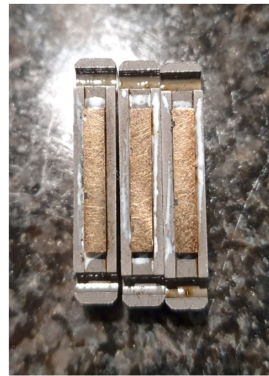
Fig. 3. cBN abrasive stones with metallic bond.
