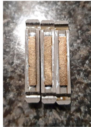
Fig. 3. cBN abrasive stones with metallic bond.
