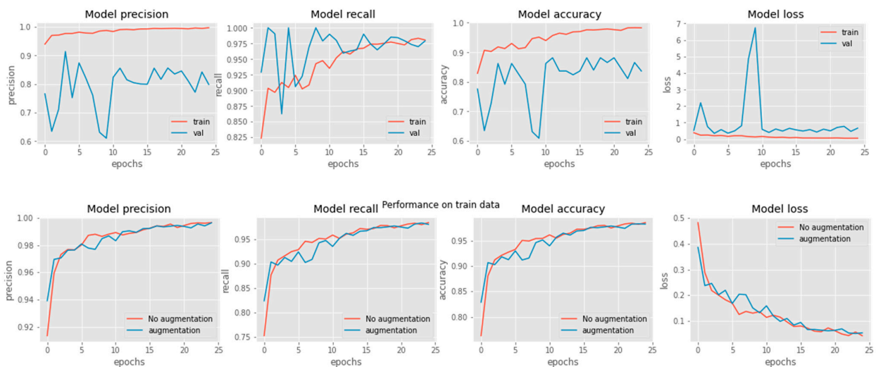
Figure 10. Comparisons graph for proposed model accuracy compared with loss related to data augmentations and no augmentation.
