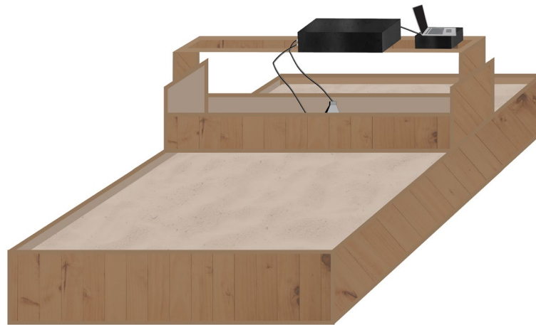
Figure 14. Illustration of the GPR configuration utilized for generating experimental training and testing data used by the proposed surrogate-assisted buried object characterization framework.
