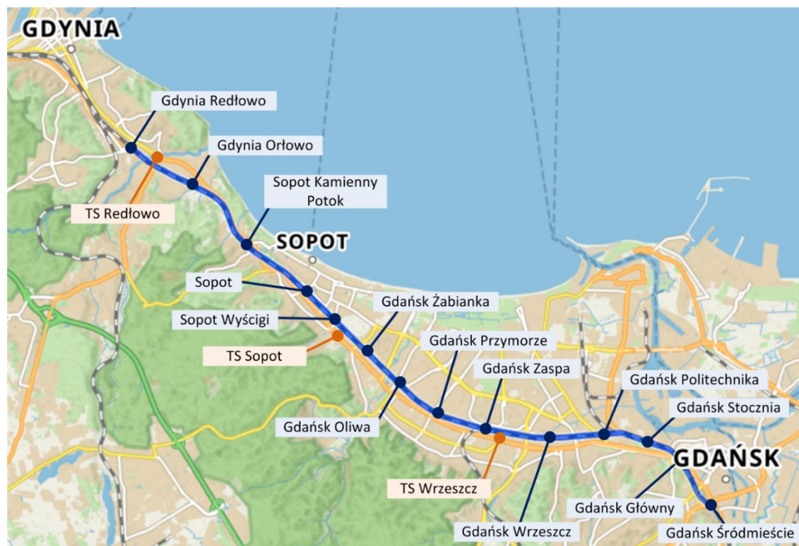
Fig. 5.2. Map of the analyzed line fragment, with stations (blue) and traction substations (orange) locations shown
