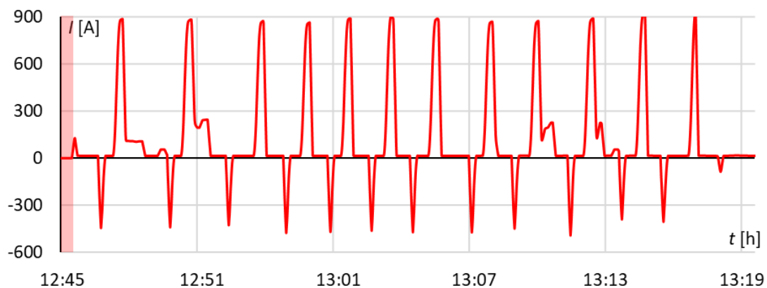
Fig. 7.11. Pantograph current optimized velocity profile – EN57AKM, track 502
