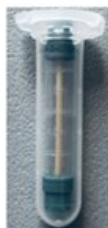
Figure S1. Both sides sealed PEEK tube placed in an Eppendorf tube.
