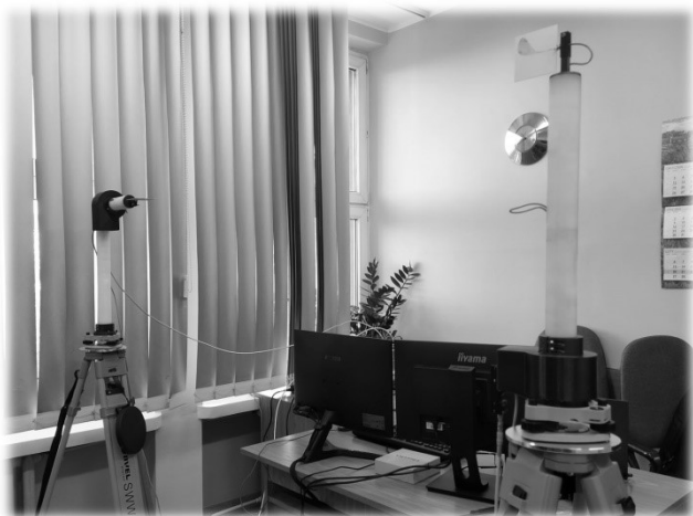
Fig. 4. Photograph of the low-cost open-hardware system for measurement of antenna far-field responses installed in the non-anechoic test site.
