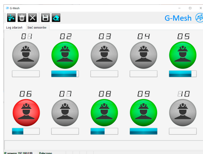
Figure 15. Interface of the G-Mesh monitoring application (gray—inactive device; green—high level of concentration; red—low level of concentration).
