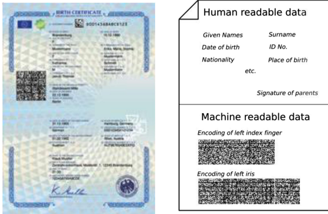
FIGURE 5 Proposed birth certificate from the FIDELITY project [46]. Left: Draft product design. Right: Sizes of barcodes correspond to the approximated storage requirement for the compressed biometric sample.
