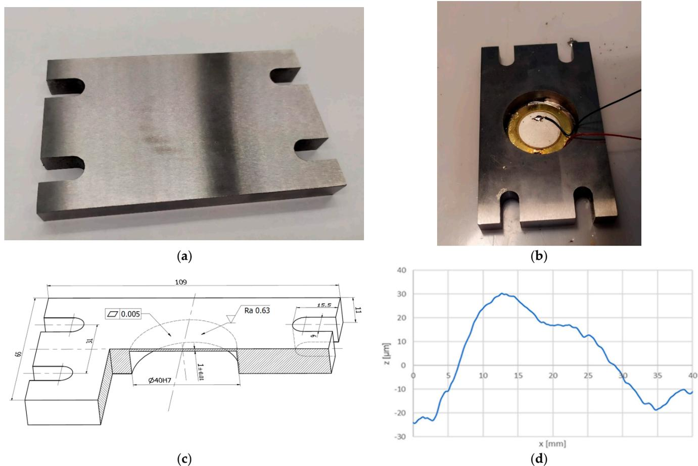
**Figure 3.** Prototype of the vibrating plate—solid block (a) view on the working surface. (b) view on the cavity with the PZT element. (c) geometry of the plate. (d) profile of the solid plate after electro-drilling.
