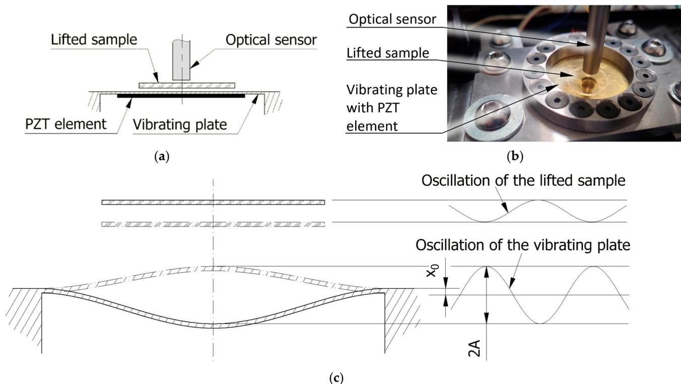
**Figure 2.** Test setup. (a) schematic view. (b) picture of the setup. (c) idea of the squeeze film lifting effect, where  $A$  is an oscillator vibration amplitude [ $m$ ], and  $x_0$  is a mean deflection of the oscillator [ $m$ ].
