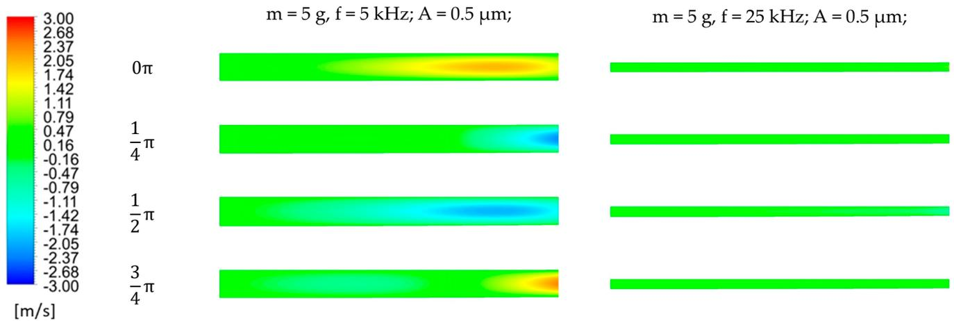
Figure 15. Fluid radial velocity contours for cases  $m = 5\text{ g}; f = 5\text{ kHz}; A = 0.5\ \mu\text{m}$  and  $m = 5\text{ g}; f = 25\text{ kHz}; A = 0.5\ \mu\text{m}$  (air thickness increased proportionally  $\times 50$  to improve the readability of the drawing).
