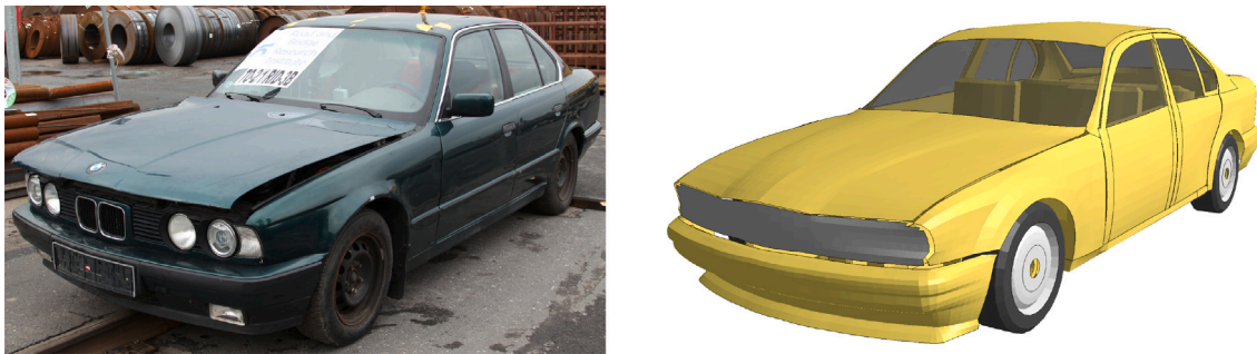
Fig. 3. Comparison between the vehicle and its corresponding numerical model.
