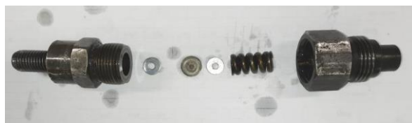
Fig. 7. Preview of injector parts which were used in the tests, among them exchangeable (adjustable) shims under the injector spring
