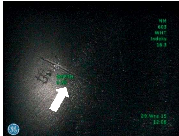
f) Measurement of the scratch depth on the piston crown made by the 'Shadow' method – 0.35 mm, with an accuracy index of 16.3, corresponding to an absolute error of 0.1 mm
