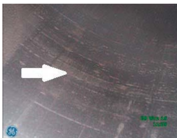
b) Cylinder sliding surface in the vicinity of BDC – traces of abrasive wear, no traces of the liner 'honing'
