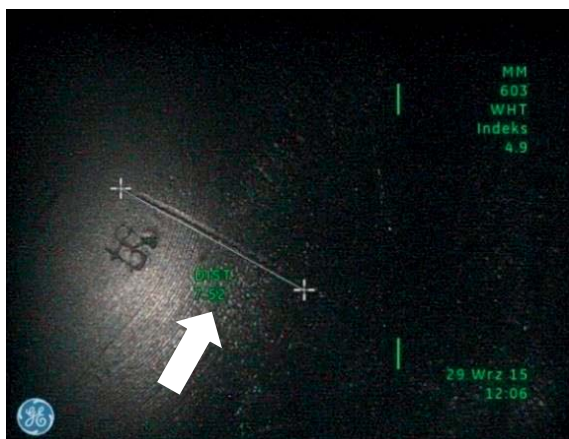
e) Measurement of the scratch length on the piston crown made by the 'Shadow' method – 7.52 mm, with an accuracy index of 4.9, corresponding to an absolute error of 0.3 mm
