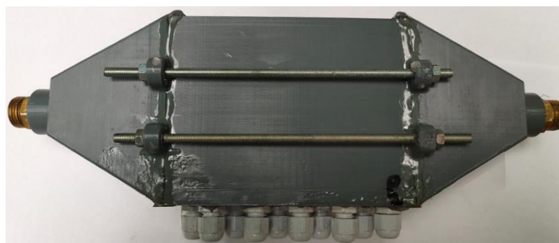
Figure 10. View of the 3D-printed heat exchanger.
