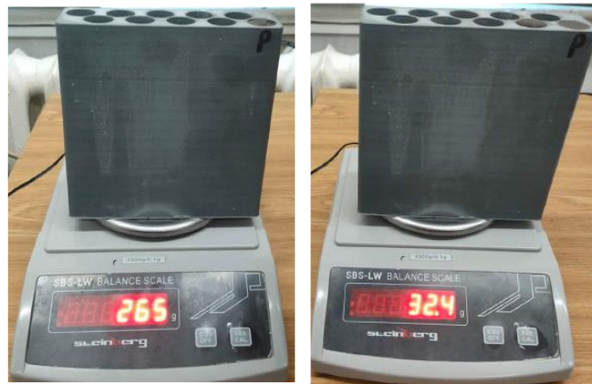
Figure 14. Weighing water after charging: cell 1 (left) and cell 2 (right).
