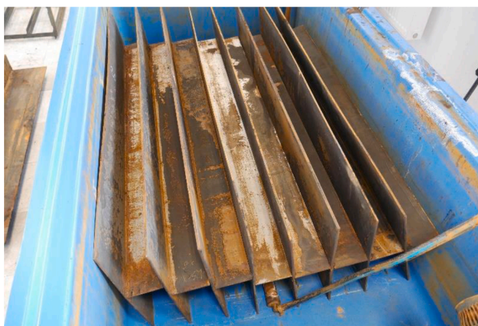
Fig. 2. Corrosion test tank (Woloszyk et al., 2021b) (1- linear diffuser, 2 – aeration pump, 3 - heaters, 4 – circulation pumps) (left) and corrosion tank with placed specimens (right).
