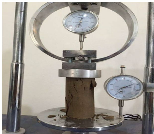
Figure 4. Specimen image after the UCS test.
