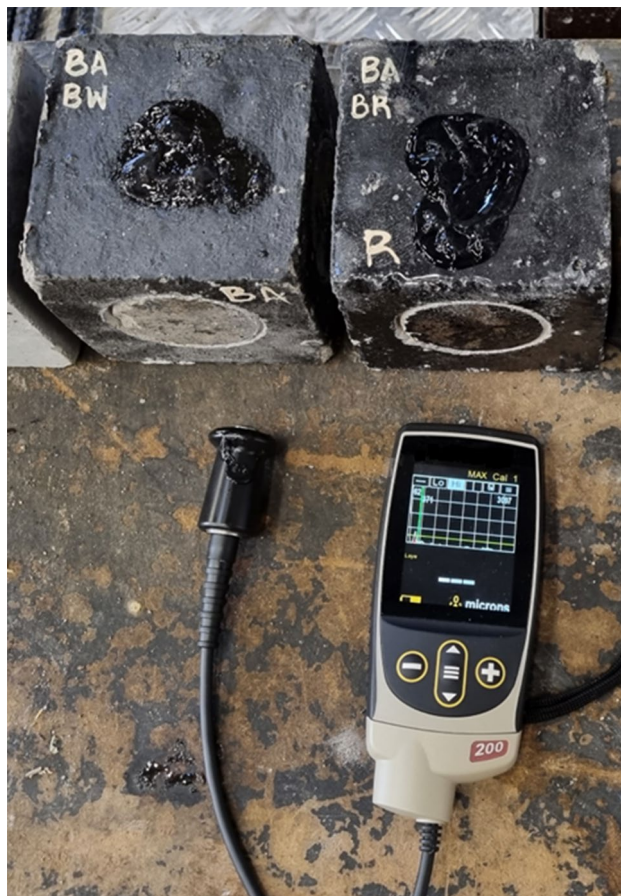
Figure 3. Measurement of coating material thickness.
