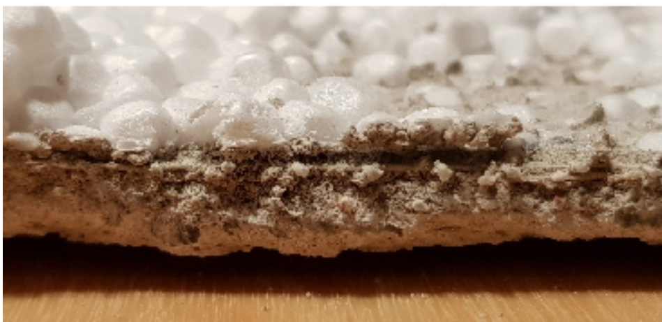
Figure 2. Details of thermal insulation (substrate) a), b) and c) for the ceramic cladding of the building facade
