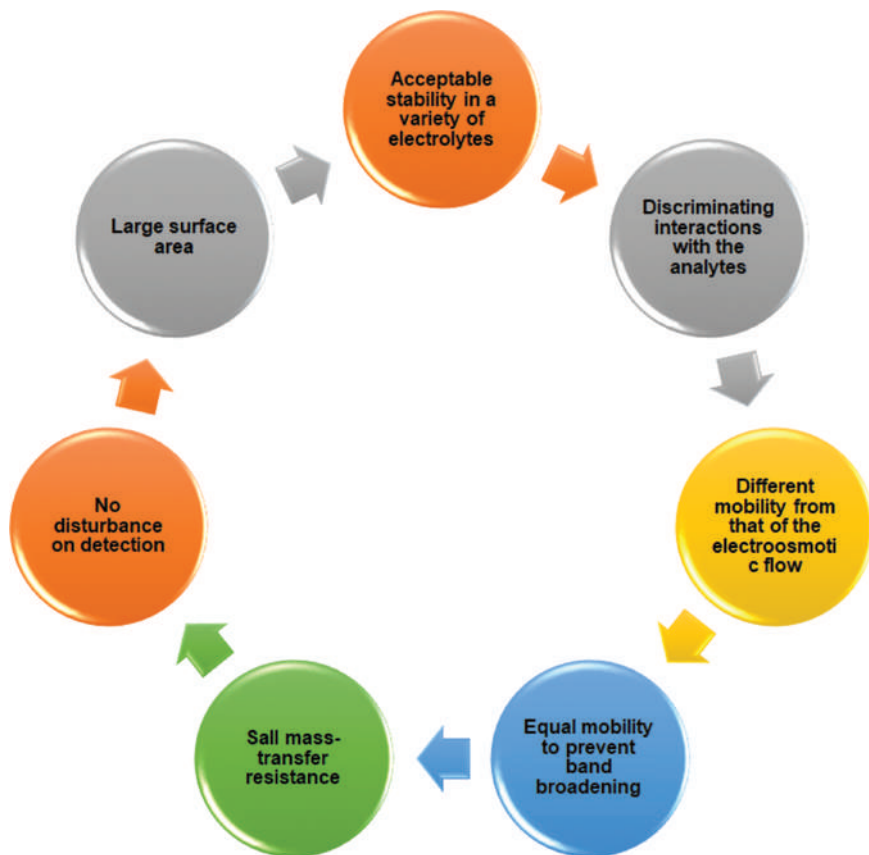
Figure 1.14 Basic requirements for nanoparticles to be used in CE (based on ref. 120).
