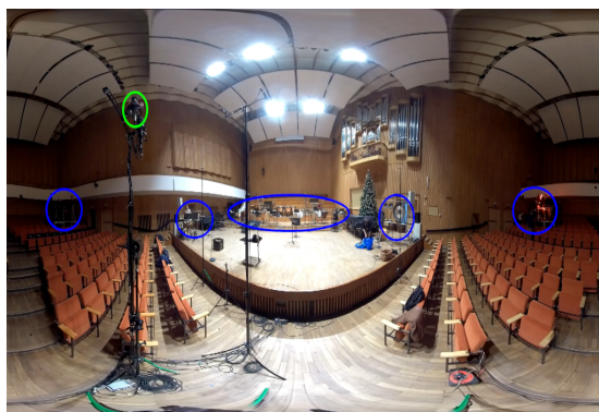
Fig. 2: Ambisonic microphone (green) and spot microphones / individual instrument zones (blue) during the second concert at the Chopin University of Music. The 360 camera is the source of the photo and thus is not visible
