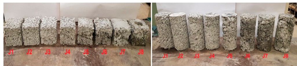
Figure 3. Cubic and cylindrical samples prior to tests—for J1–J8 mixes see Table 4.
