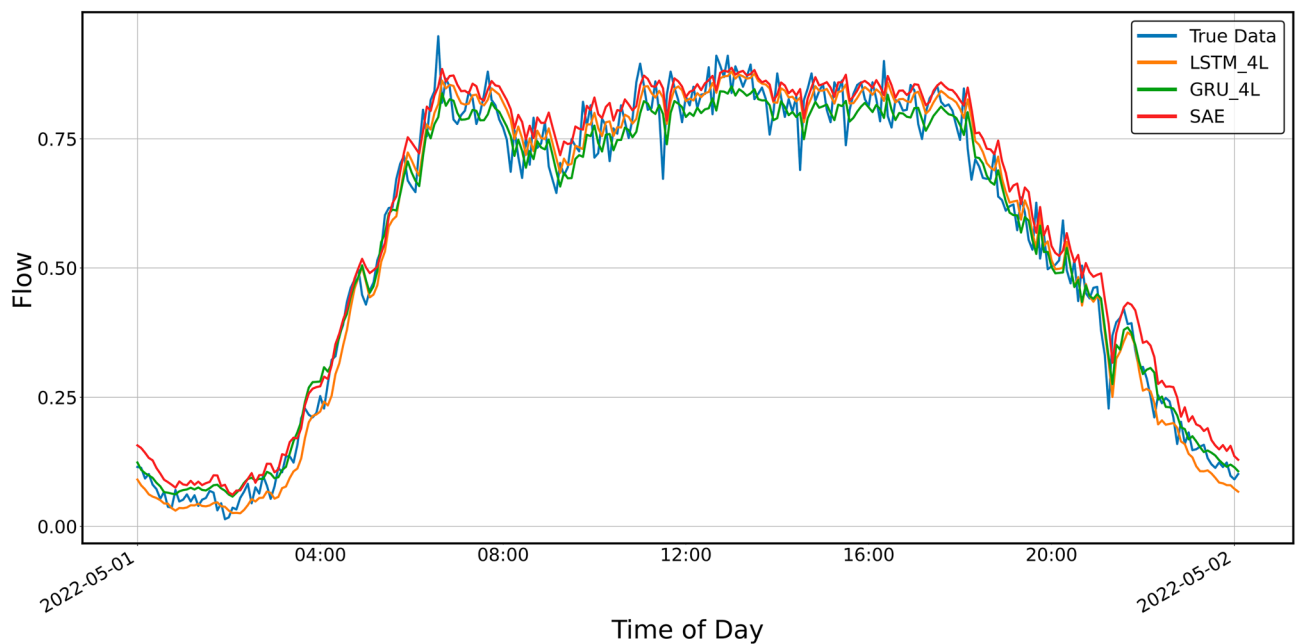
Figure 14. Prediction result for SAE and 4-layer LSTM and GRU models, prediction period 24 h.
