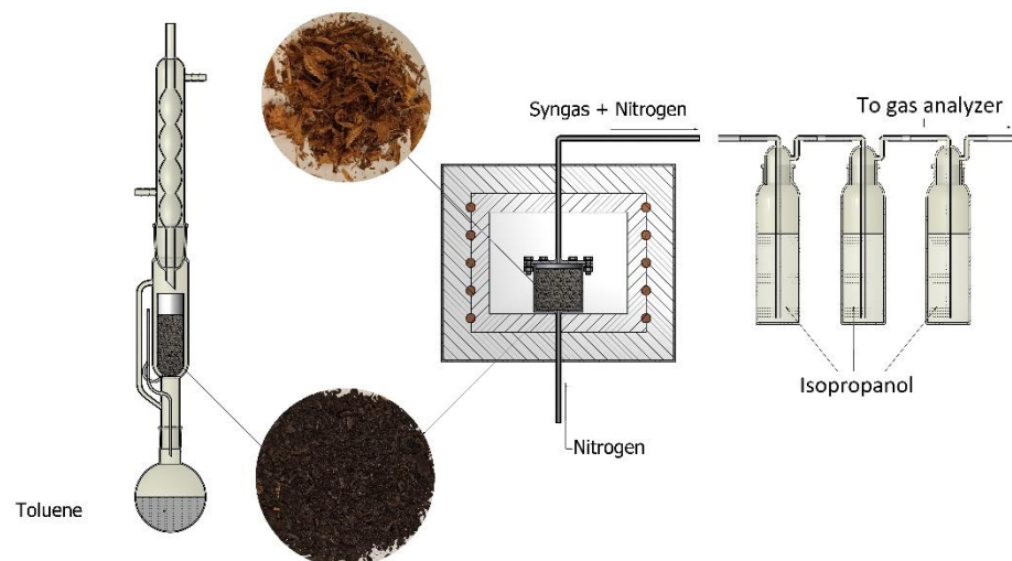
Figure 3. Scheme of the experimental setup for thermal neutralization of waste.
