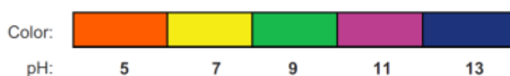
Fig. 4. Concrete discoloration chart for the control liquid - Rainbow Test (based on materials from Germann Instruments)
