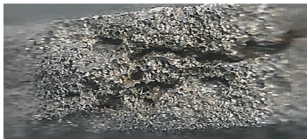
Fig. 1 Image of the corrosion coupon surface after exposition in the aqueous environment with H 2 S
