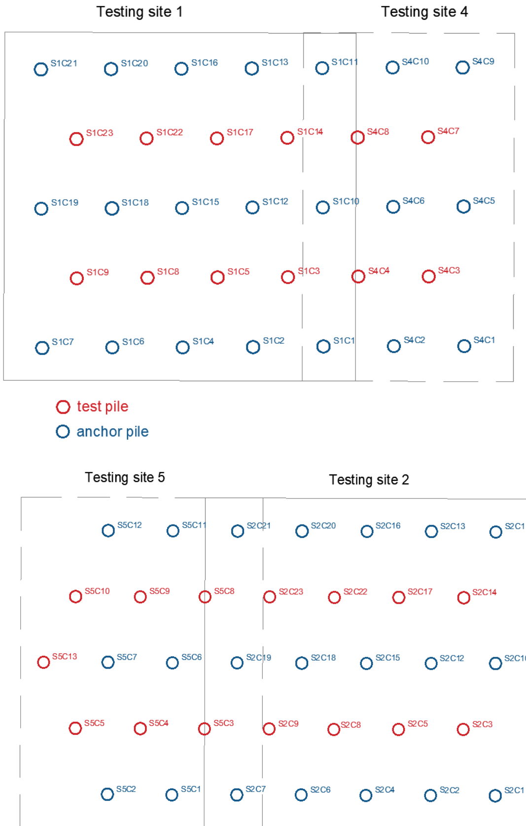
Figure 5.2. Arrangement of columns on testing sites
