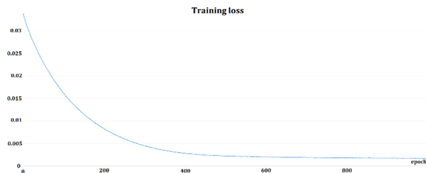
Figure 6. Example of training loss function for Deep Speaker model triplet-loss training.
