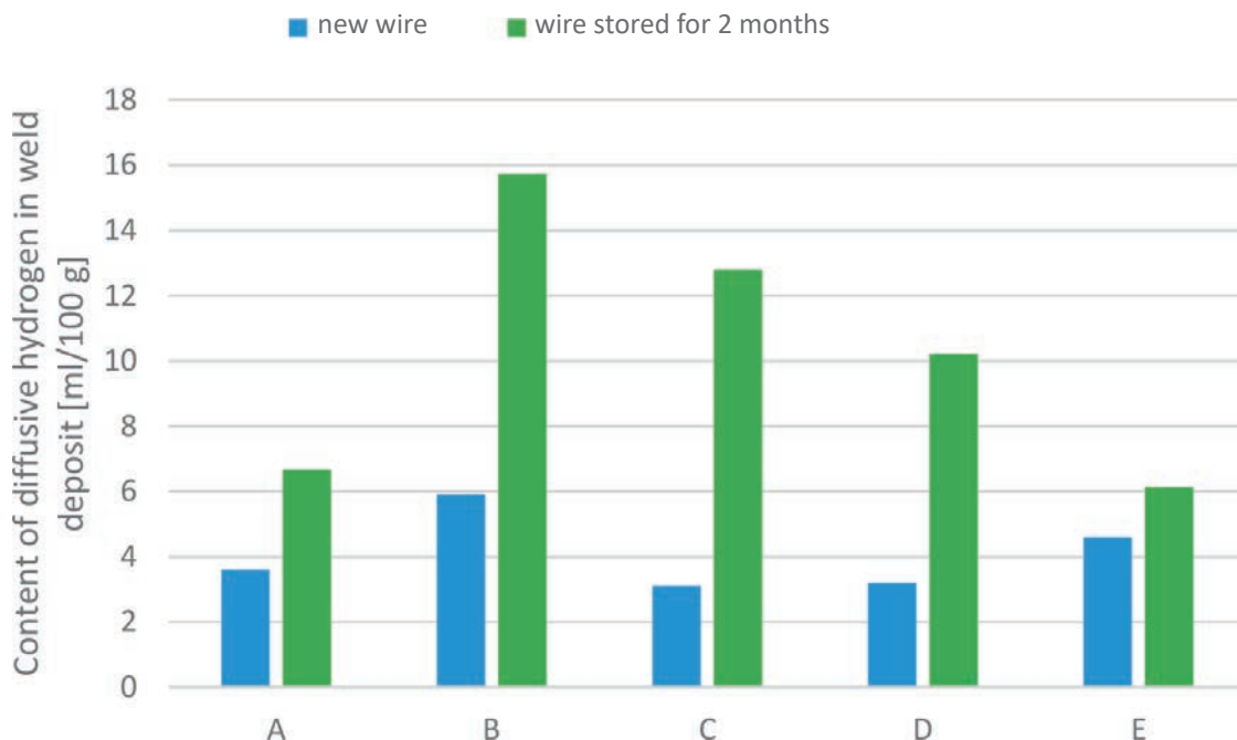
Fig. 7. Content of diffusive hydrogen in the weld deposit in relation to new and stored flux-cored wires
