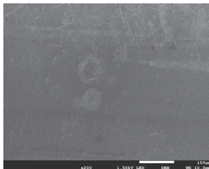
Fig. 3. Photograph (SEM) of the copper-clad wire surface
