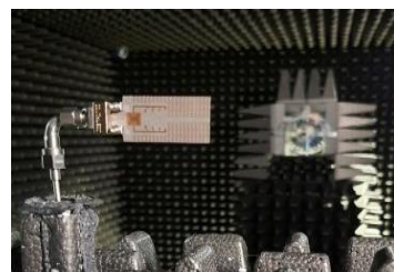
Figure 12. The radiation pattern measurement setup.
