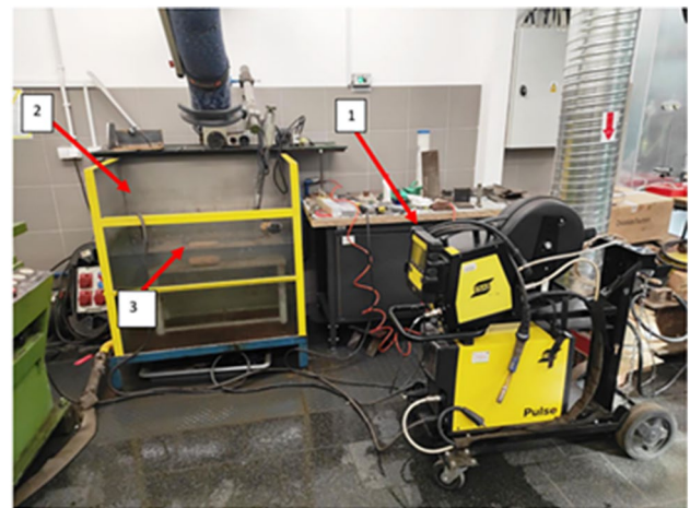
Fig. 1 The welding stand: 1—welding power source and wire feed unit, 2—tank, 3—welding table
