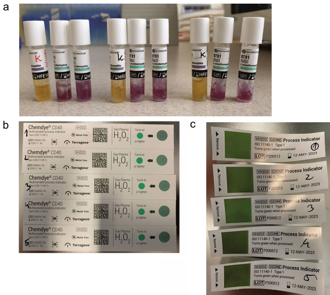
Figure 1. Quality controls used in the study. (a) Standardized biological quality controls containing G. stearothermophilus (ATCC7953) spores with CFU 1.3 \times 10^5 and a liquid culture medium with a color indicator (additionally equipped with chemical strips to indicating exposure to H_2O_2 vapors). Vials that were not sterilized are labelled with “K” (yellow medium indicates bacterial growth) and vials after completing the sterilization process show a violet color (indicating a lack of bacterial growth). (b) Chemdye CD40 type-4 commercial chemical tests strips confirming the effectiveness of the H_2O_2 vaporization (test field colored green) in the tested sterilization station. (c) VH2O2 Process Indicator strips type-1 confirming the effectiveness of the H_2O_2 vaporization (test field colored green) in the tested sterilization station.
