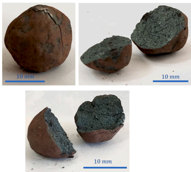
Fig. 11. Pellets aspect after the compression tests.
