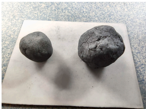
Fig. 13. Pellets reduced in hydrogen at 1000 °C.
