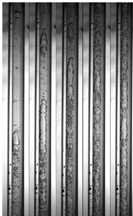
Figure 8. Flow Patterns Pr=0,6 G=180 kg/(m 2 ·s) Quality respectively: 37,2%, 48,6%, 64,6%, 72,8%, 93%
