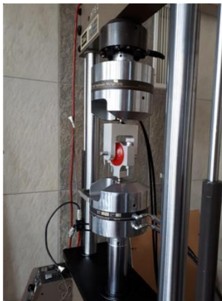
Figure 3 Specimen during fatigue test (80 ShA)
