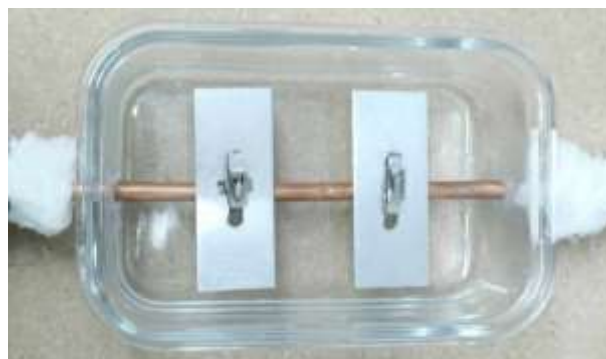
Fig. 2. Aluminum fins added inside PCM container.
