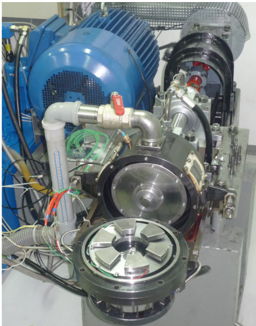
Fig. 2 Photograph of the bearing test rig with an open cover showing the front test bearing.
