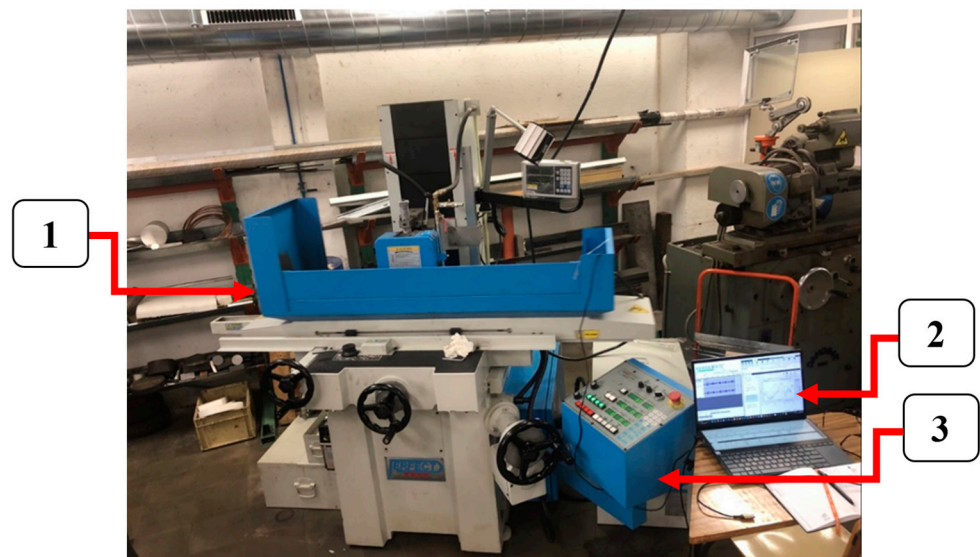
Figure 1. Tangential grinding machine used in the experiments: 1—CNC grinder, 2—computer with Matlab and Audacity software, and 3—control panel of the CNC grinder.
